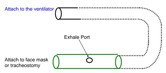
The circuit comprises of a 22mm wide reusable tube for the patient output about 1.8m in length shown here in black. With a connector at the patient end containing an opening or Exhale Port (Whisper swivel).
